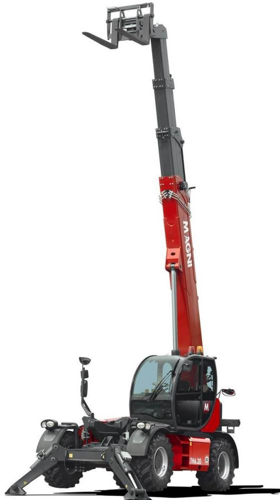
With rotating units from 8m to 24m lifting height, the TH range comes with 5 tonne to 6 tonne capacities: 5.5 tonnes lifting capacity, 15m lifting height; 5.5 tonnes capacity, 19m height; 5.5 tonnes capacity, 24m height; 6 tonnes capacity, 10m height; 5 tonnes capacity, 8m height; and 6 tonnes capacity, 20m height.
