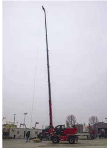
the management of the stabilizers proportional so as to guarantee a millimeter leveling even in the most demanding conditions. Thanks also to the RFID system which provides automatic recognition and creation of the dynamic load charts; this telescopic handler is able to meet a wide range of applications in construction and industry.
